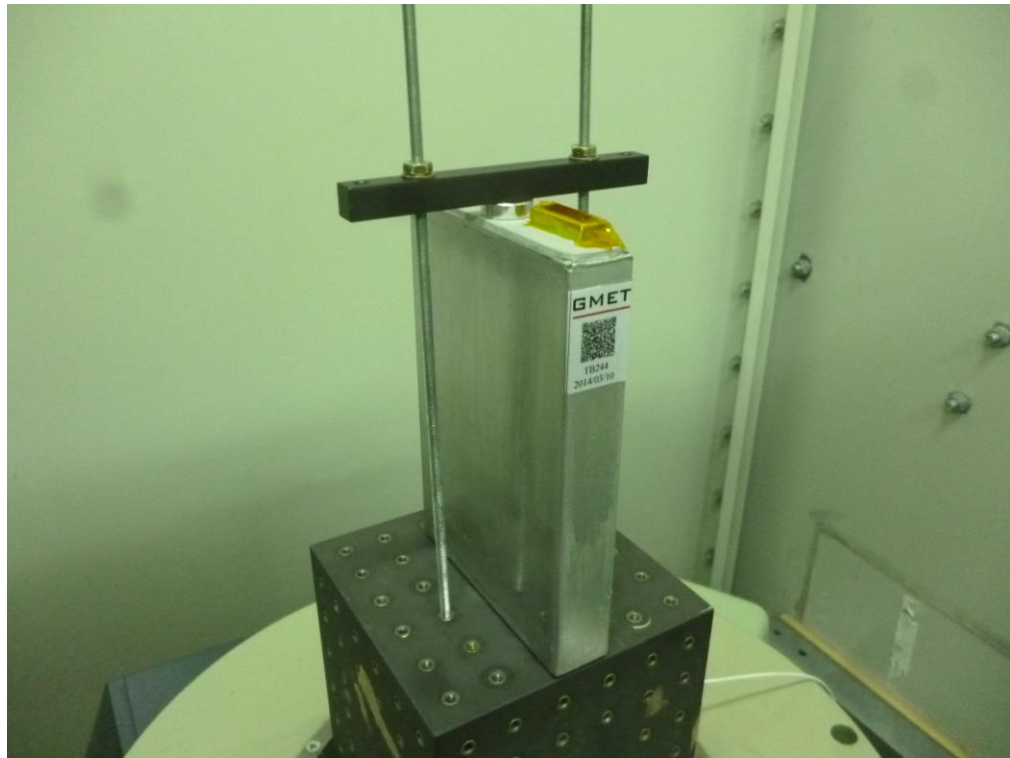
Vibration test condition -1 (X axis direction)
